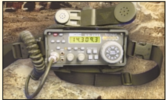
Photo A— The SG-2020 ADSP 2 works the same as the basic SG-2020 except that the internal ADSP 2 board adds interfering carrier attenuation, atmospheric noise-fighting capability, and bandwidth filter.
